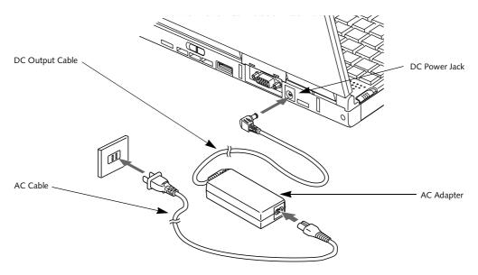
Figure 3-1 Connecting the AC Adapter
